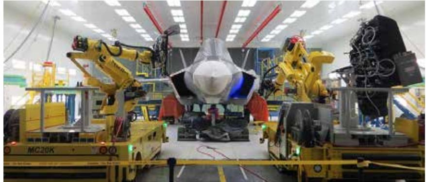
**THE AIR FORCE HAS A ROBOTIC SYSTEM CAPABLE OF RESTORING THE SPECIAL COATINGS ON AN F-22'S AIR INLET DUCTS MORE QUICKLY AND CHEAPLY THAN DOING SO BY HAND.**
